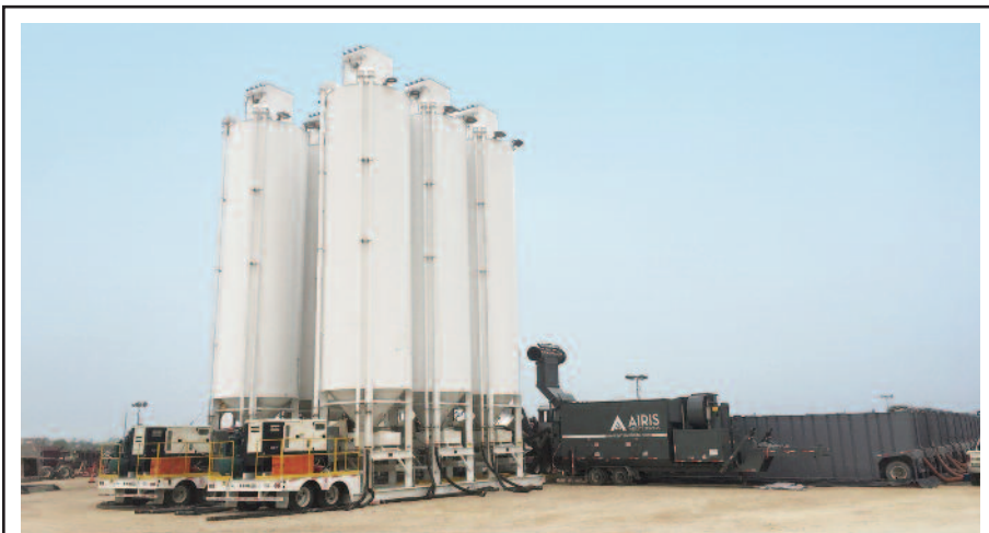
To meet the Occupational Safety and Health Administration's limit on employees' exposure to respirable crystalline silica, AIRIS Wellsite Services generally recommends installing vacuums around sand transfer points to capture dust before it can reach employees. The company cites years of data showing that vacuums work well and have a minimal effect on operations.
