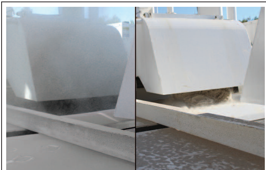
By replacing traditional silica sand (left) with sand that has been treated to minimize dust formation (right), employers can reduce their workers’ exposure to respirable crystalline silica below the triggering point for burdensome regulations, Covia reports. The company describes the treated sand as affordable and effective.
