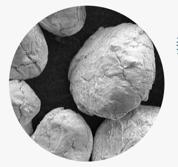
LUMINEX begins as strong, rounded Northern White sand grains that are thermally processed.
