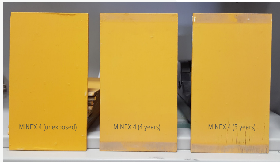
Figure 2. Visual comparison of unexposed MINEX 4 control with four and five year MINEX 4 test panels returned by Q-Labs.
