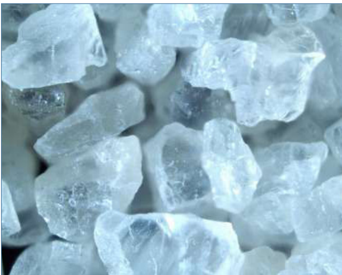
Figure 2. Reflected and transmitted illumination photomicrograph of liberated nepheline syenite grains from the ore.
